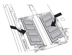
Figure 8-14 Installing two memory modules
